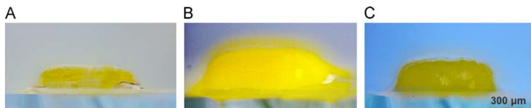
Fig. 4. Photo-switchable ionogel after photopolymerisation (A), swelling in 1 mM HCl for 2 h (B) and shrinking upon white light irradiation (C).
